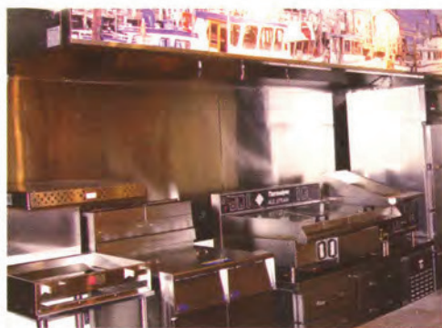
At Bello Pronto, equipment includes a convection oven, a gas six-burner cooktop with refrigerated drawers beneath, two pasta cookers, three panini grills, a humidified hot food cabinet, a heated granite shelf and a drop-in ice pan.
